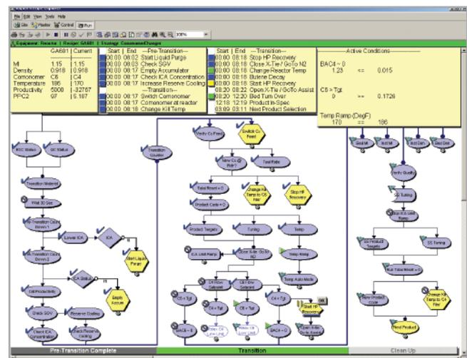
The Sequence Control features of aspenONE integrate operator actions with the control application. Operators can view the task list and see progress indicators for each task.
